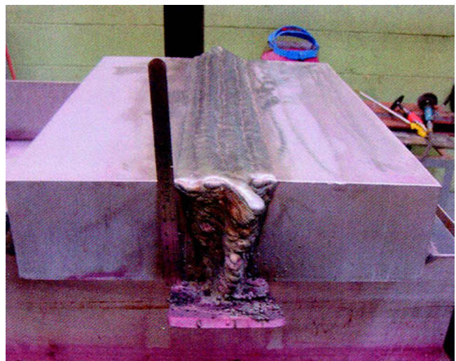
Fig. 11 End view of a completed 7.5 cm (3 in.) thick Haynes 230 alloy weld. Source: (Ref 16)
